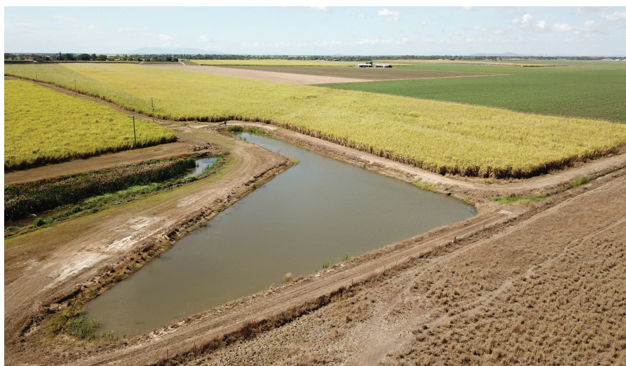
Mugica Farm water recycle pit – to capture and re-use run-off water
