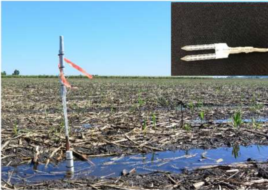
A sensor has been installed at the top of the block to record irrigations:
