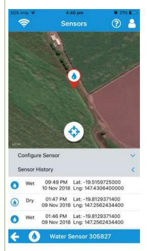
That being said, there were some readings that came through that didn't make a great deal of sense and this reduced the growers confidence in the sensor. The example below is an indication of these incorrect readings. In this case, the sensor state change from wet to dry to wet 3 times between 5:30am and 11:30am. These changes of state may have been due to the float switch moving with waves in the water (instead of reacting to a change in water height).
