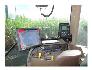
A GPS unit and fertilizer flow rate controller inside the
