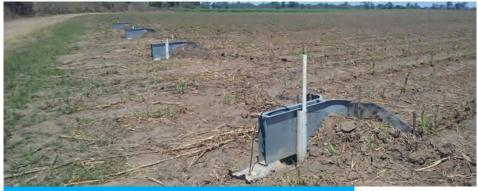
*Above:* Auto flumes at Ayr Farming Project Catalyst site measuring runoff flux (volume x concentration)
