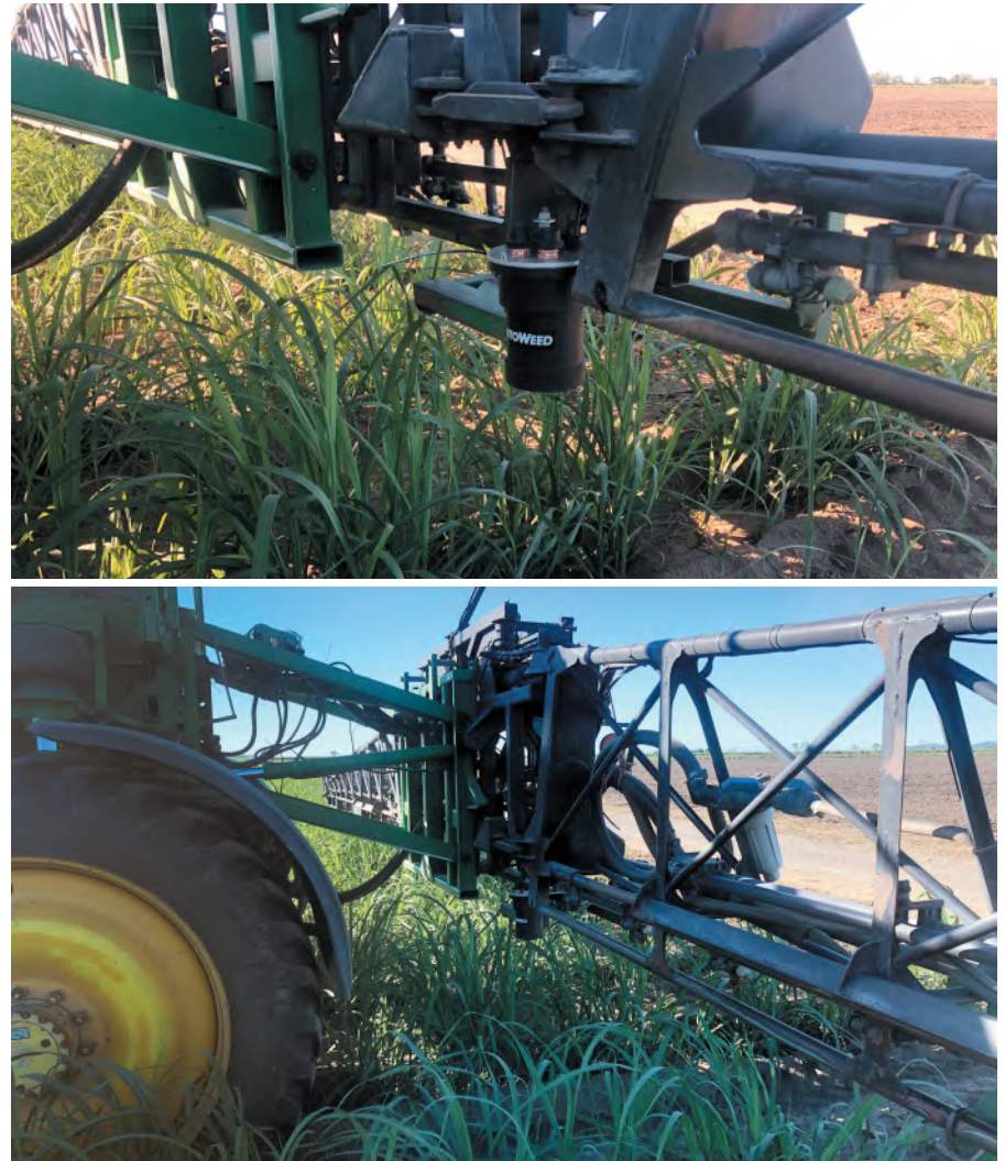
Figure 5 - AutoWeed Irwin leg mount retrofit designed for a John Deere 4720 self-propelled sprayer
