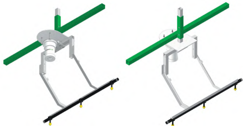
Figure 5 - AutoWeed Irwin leg mount retrofit designed for a John Deere 4720 self-propelled sprayer
