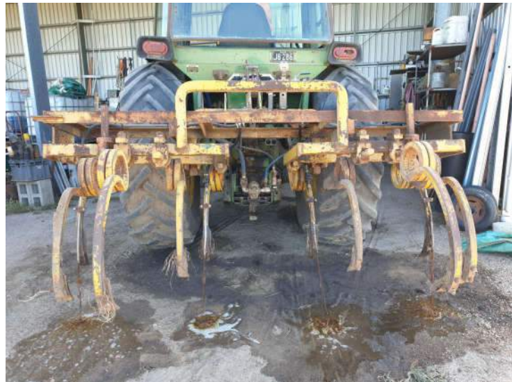
Calibration of molasses applicator
