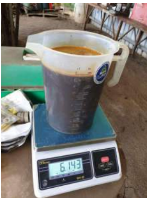
Molasses density being measured
