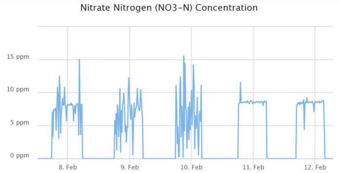
The above data shows a number of irrigation events that have occurred following the sensor installation. The block is split into 5 sets which is the reason for 5 separate readings. As can be seen in the first 3 irrigations, there is significant turbulence in the readings (0-16mgNO3-N/L); however when the raw data is exported, the mean and the median value are very similar to the second two events where the readings are far more stable (approx. 8mgNO3-N/L).
