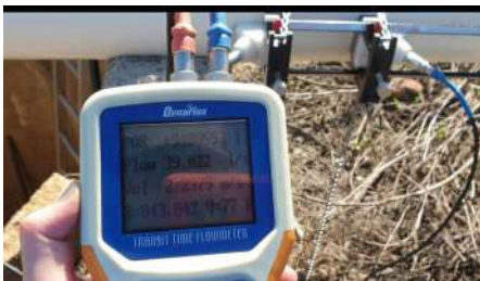
Performing a pump flow assessment on a bore using an ultrasonic flow meter
