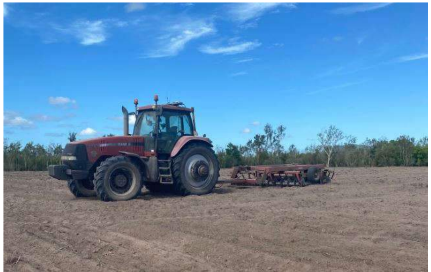
Fig.3 Controlled traffic tractor pulling off-set equipment
