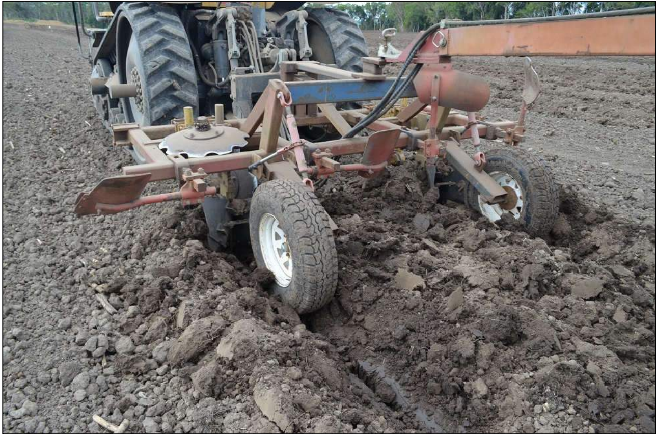
Figure 6 - Ameliorants including mill mud and ash are banded into the furrow
