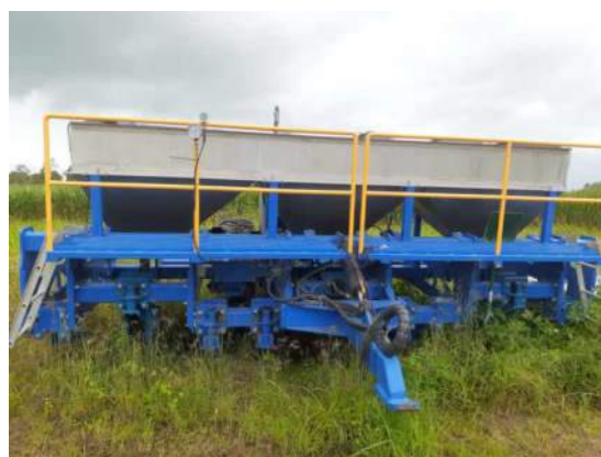
Fig.2 The Fox's fertiliser box which allows for variable rate N application
