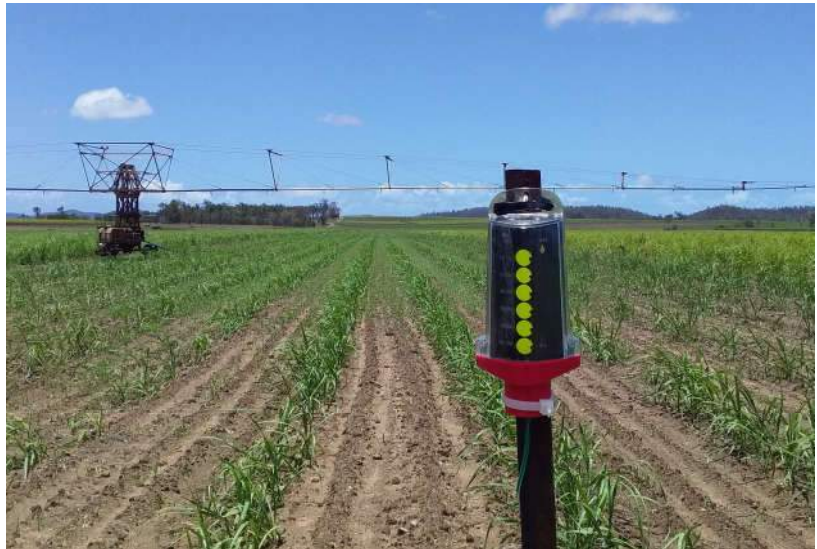
Fig.3 Soil moisture probe (GDot) in plant cane following oat crop
