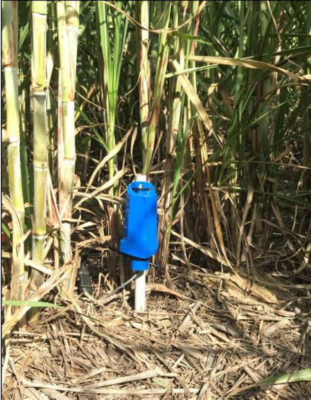
*Figure 4 - Wireless moisture sensor*
