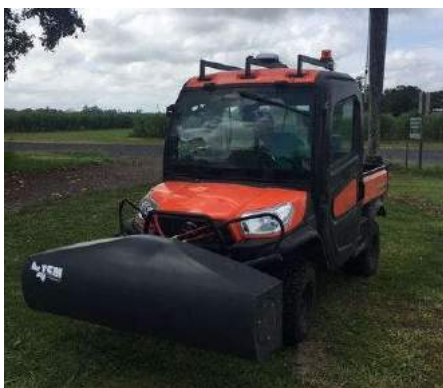
Fig.4 Topsoil mapper (TSM) used by Farmacist to identify variability & constraints.
