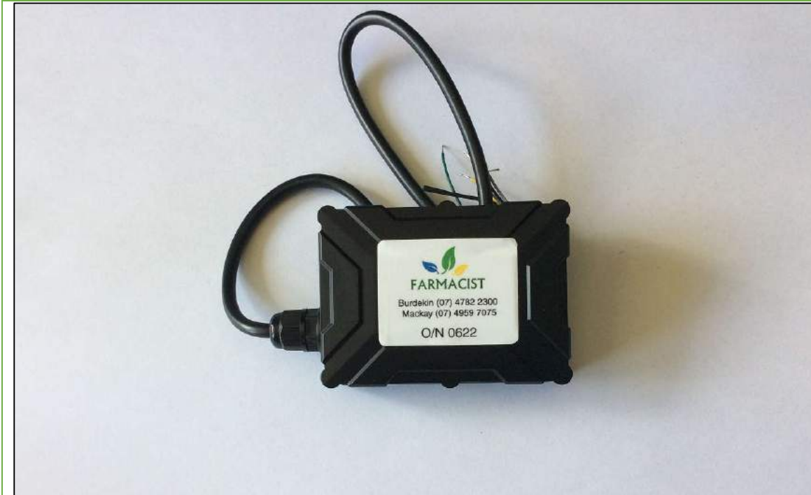
Figure 8 - Upgraded GPS monitor fitted to the harvester for the 2019 harvest season.
