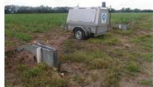
CSIRO's set up which is monitoring the quality of runoff from the trial site
