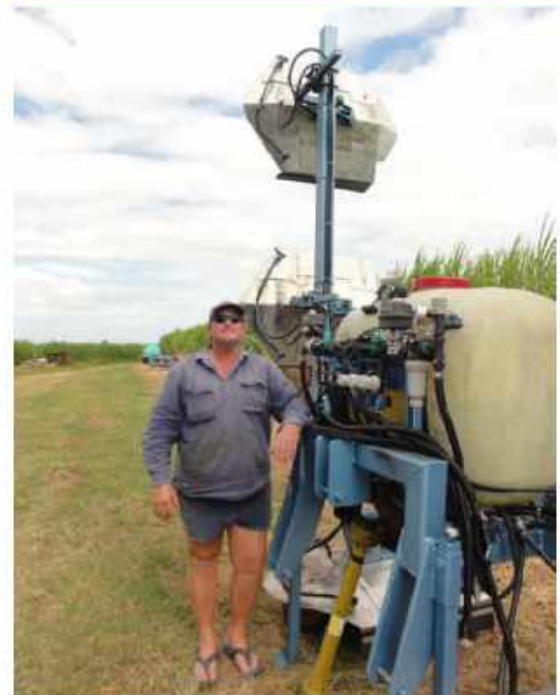
Dennis with his variable rate shielded sprayer
