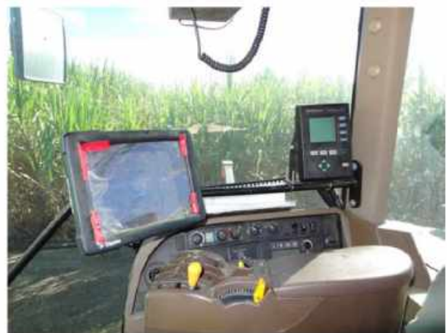
A GPS unit and fertilizer flow rate controller inside the tractor
