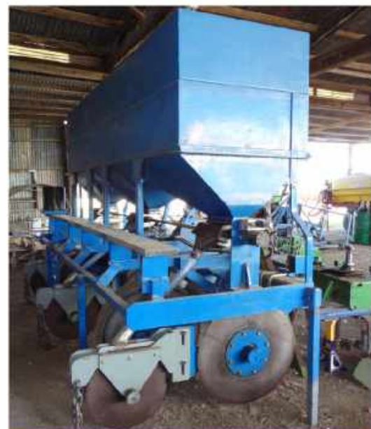
A sub-surface fertilizer box places nutrient in the crop's root zone.
