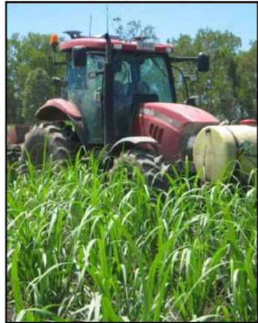
Tractor showing GPS roof array and front tank where the Confidor Guard is carried.
