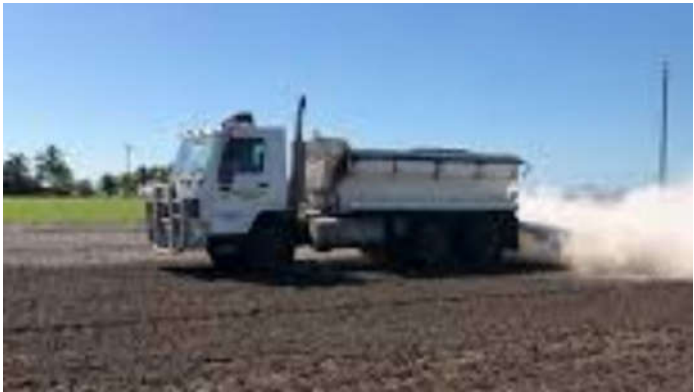
Gypsum Spreader addressing Soil Constraints of Cracking Clay Soils
