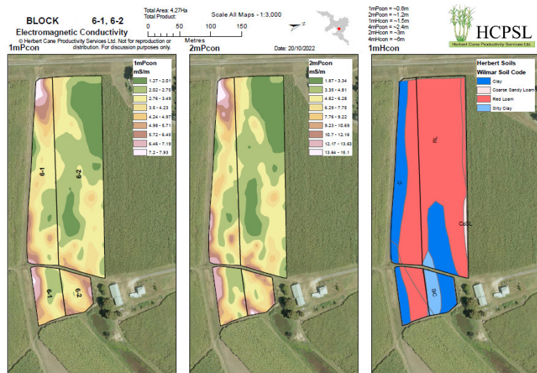
EM and Soil Map displaying soil variability readings influenced by moisture & constraints
